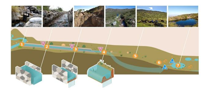
Conceptual representation of how the pre-Inca infiltration system works. Water is diverted during the wet season using canals that transport surplus water during the wet season to high permeabilityzones. Water penetrates the soil and emerges in downstream springs after weeks or even months, which provides water during the dry season. Credits: Ochoa-Tocachi et al., Nat. Sustain., 2019.
