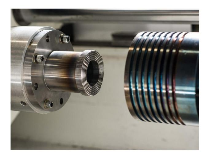
PNNL's ShAPE<sup>TM</sup> process combined with a unique aluminum alloy produced high-strength, high-ductility rods in one single process. Credit: Andrea Starr | Pacific Northwest National Laboratory
