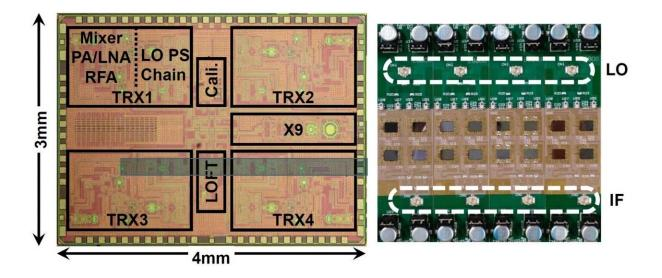
The transceiver, based on a 64-element phased-array design, takes up a chip area of  $12 \text{ mm}^2$ . Credit: IEEE
