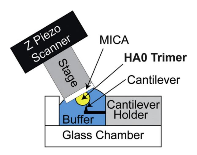
HS-AFM setup for direct visualization of HA0 trimer. Schematic diagram of the HS-AFM setup for scanning the HA0 trimer. Credit: Kanazawa University
