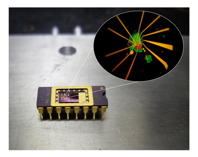
A Hall-bar device structure (see inset) is wire-bonded to a 16-pin chip-carrier. The chip-carrier allows for extensive electrical characterization of the device at both low temperatures and high magnetic fields. Credit: Min Sup Choi/Columbia Engineering
