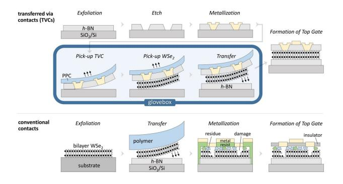
The fabrication process for transferred contacts that yield nearly ideal transistors. Transferred contacts prevent contamination and damage to the 2D semiconductor that occur during fabrication of conventional contacts. Credit: Min Sup Choi/Columbia Engineering
