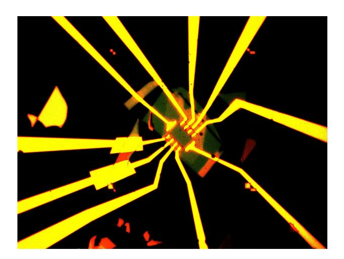
An enhanced optical microscope image of a Hall-bar structure used to characterize transistor properties for devices made with ultraclean transferred contacts. The long radial lines, made from deposited gold, connect the small contacts at the center of the device to large probe pads for easy measurements. Credit: Min Sup Choi/Columbia Engineering
