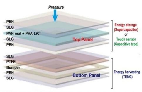
SLG (Electrode), PEN, PTFE (Flexible substrate, Triboelectric surface)
