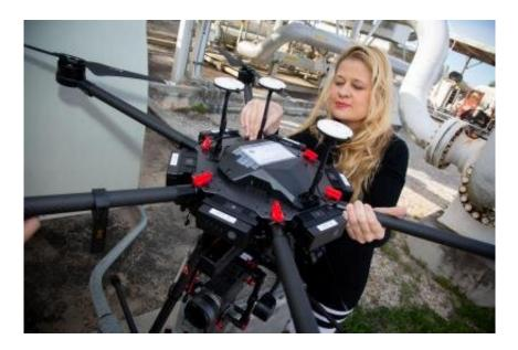
Maria Araujo inspects a drone that uses midwave infrared cameras (MWIR) to autonomously detect methane leaks. SwRI's Smart LEak Detection System (SLED) uses computer vision and machine learning to detect pipeline leaks from aerial drones. Credit: Southwest Research Institute
