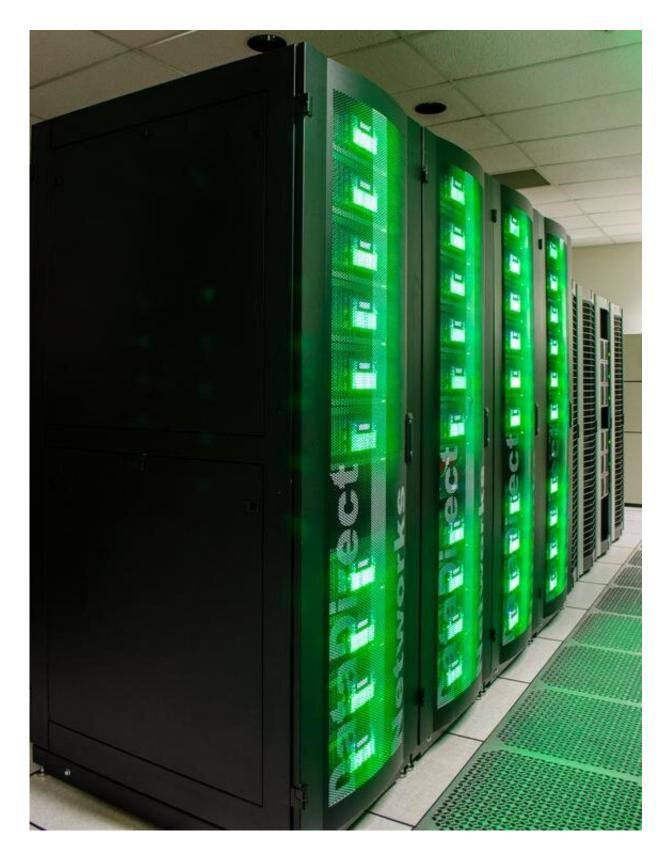
Ranch upgraded to the DDN SFA14K DCR block storage system, supplied by
