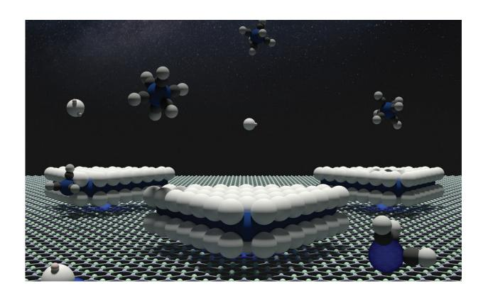
Graphic showing a boron nitride surface with tungsten atoms anchoring triangular domains illustrating defect control of the orientation. Credit: Xiaotian Zhang/Penn State
