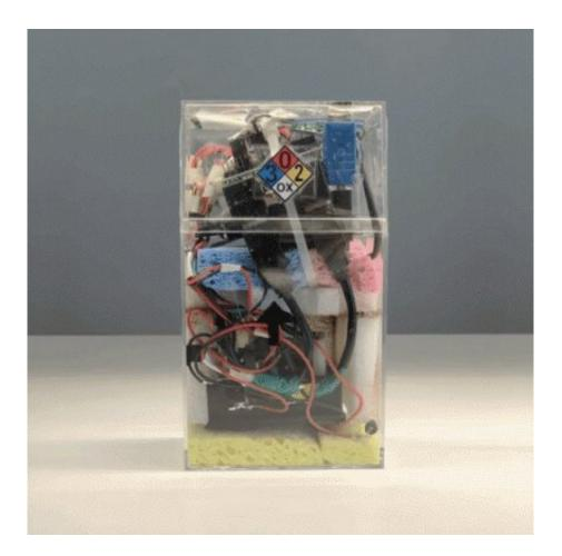
Self-contained nanolab sent for a microgravity experiment in the rocket. Credit: Harpreet Sareen, Anna Garbier, Jiefu Zheng
