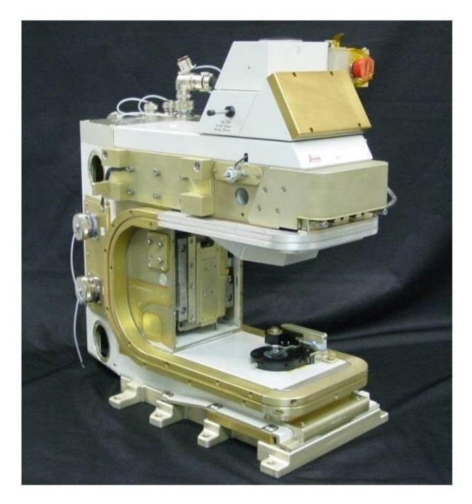
The Light Microscopy Module (LMM) enables novel research of microscopic phenomena in microgravity, with the capability of remotely acquiring and downloading digital images and videos across many levels of magnification in 3D using confocal microscopy. Credit: NASA
