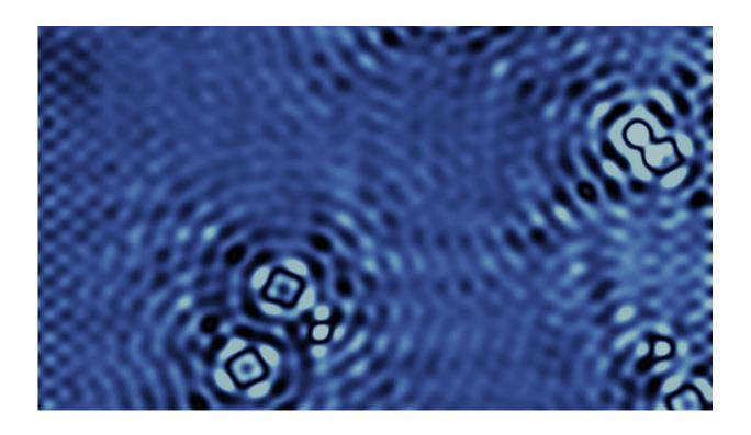
Interference of electron waves on the surface of a material, as measured with the scanning tunneling microscope. The waves form when electrons scatter off surface defects, which are visible as brighter features in the image. Credit: Irene Battisti
