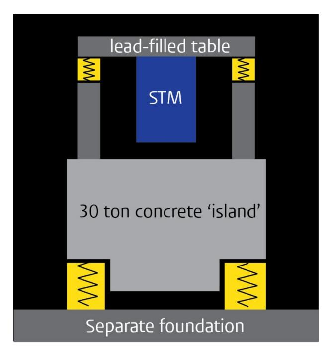
A schematic view of the set-up. Credit: Battisti
