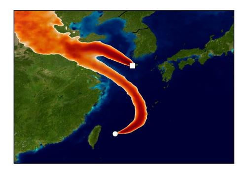
Simulated atmospheric transport of CFC-11 to the Gosan and Hateruma monitoring sites using the Met Office NAME model. The colours show areas where emission sources would strongly impact the CFC-11 measurements for one day in December 2014. This model information has been used to infer a rise in emissions from eastern China, starting around 2013 Credit: University of Bristol
