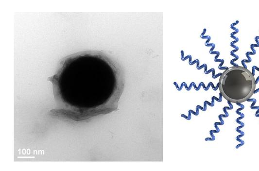
Left: A single liquid metal nanodroplet grafted with polymer chains. Right: Schematic of polymer brushes grafted from the oxide layer of a liquid metal droplet. Credit: Carnegie Mellon University
