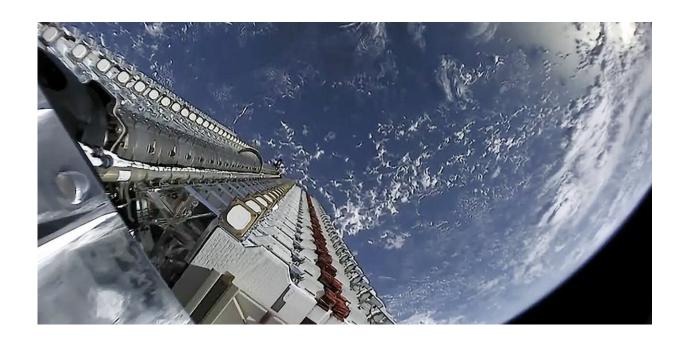
The panel of 60 Starlink satellites just before they were released to go into orbit around Earth. Credit: Official SpaceX Photos
