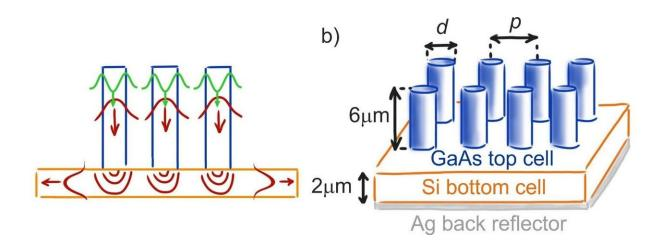
Optically coupled tandem of GaAs nanowires (6um tall) on silicon ultrathin film (2um). Sunlight is efficiently absorbed in each nanowire, and the array will transmit infrared light to be trapped into silicon film. Credit: source AMOLF
