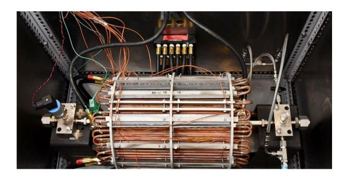
A calorimeter designed by UBC researchers that is capable of detecting anomalous heat at high temperatures and high pressures. Credit: University of British Columbia
