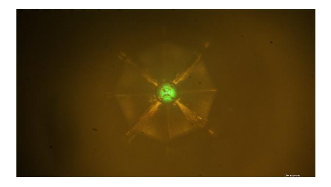
Scientists bombarded a sample of a new superconducting material with X-rays to study its structure at the Advanced Photon Source at Argonne National Laboratory. The X-ray fluorescence creates the greenish color at the sample (center). Credit: Drozdov et al.
