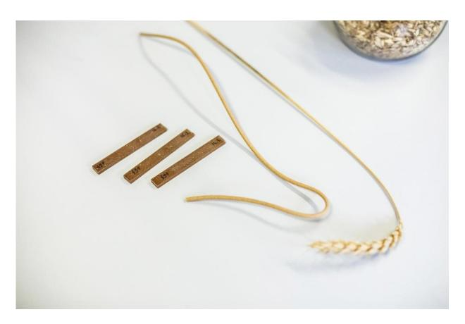
Bioplastic created at KTU laboratories is made from cellulose -- a natural material, the main building block of plant cells' membranes. Credit: KTU/Juste Suminaite
