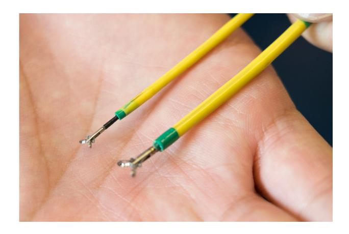
Closeup of the robotic catheter tips. Researchers are modifying them so they can be equipped with an endoscopic camera and a guidewire. Credit: David Baillot/UC San Diego Jacobs School of Engineering
