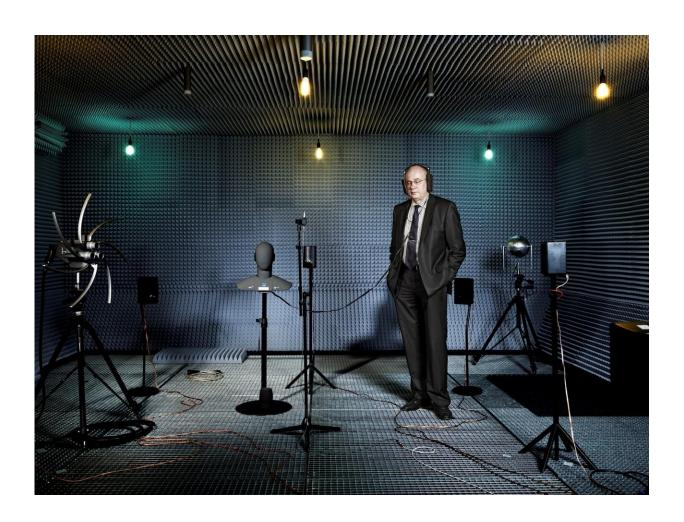
Klaus Genuit photographed in an anechoic chamber with several loudspeakers to simulate a virtual acoustical scenery, as well as an artificial head for binaural recording Credit: Genuit
