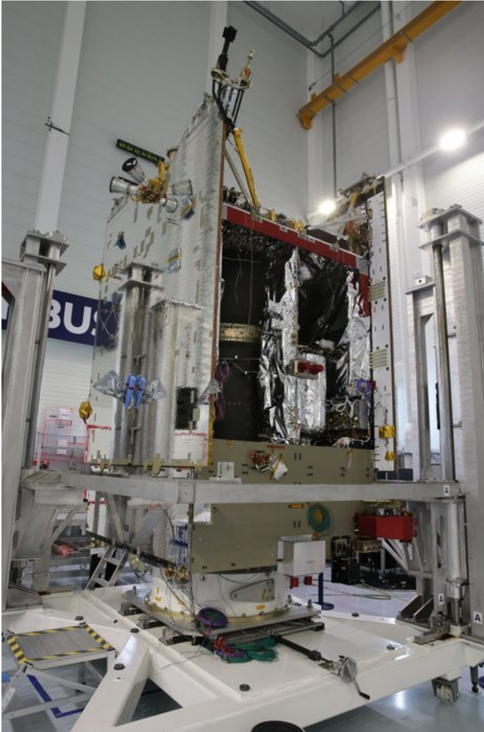
Quantum satellite after mating of payload and service module. Credit: Airbus
