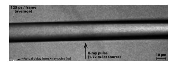
After blasting tiny jets of water with an X-ray laser, researchers watched leftand right-moving trains of shockwaves travel away from microbubble filled regions. Credit: Claudiu Stan/Rutgers University Newark
