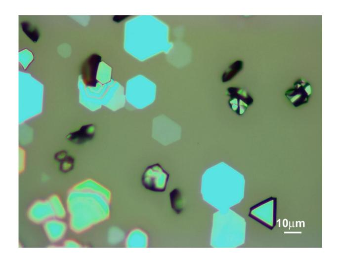
A microscope image shows flakes of epsilon-iron(III) oxide grown on mica by Rice engineers. The nearly 2D crystals are promising building blocks for electronics and spintronics that take advantage of their stable magnetic properties. Credit: the Lou Group
