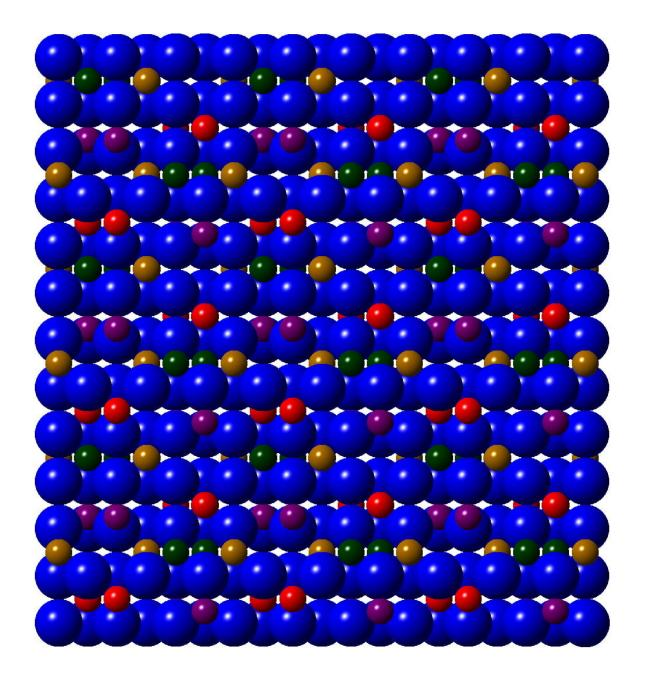
An illustration shows the structure of epsilon-iron(III) oxide, an atomically thin material that is stable, stackable and unlike other iron oxides retains its unique magnetic properties at room temperature. Credit: Jiangtan Yuan
