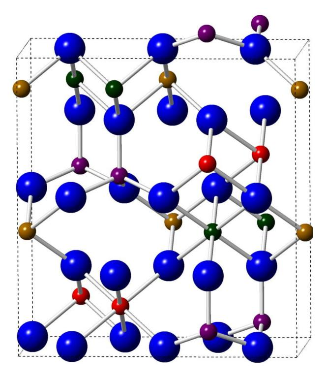
Epsilon-iron(III) oxide incorporates oxygen atoms (blue) and iron atoms (everything else) into a crystal lattice with magnetic properties that, unlike other iron oxides, remain stable at room temperature. This makes the nearly 2D material a good candidate for combining with other atom-thick materials for
