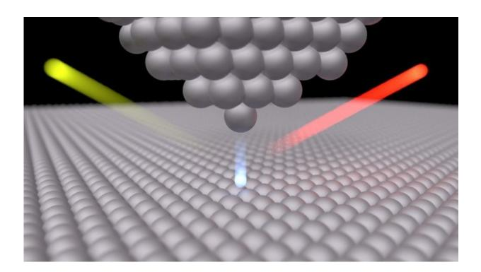
Controlled quantum signals: When electrons (light blue) tunnel from the tip of a scanning tunnelling microscope to a sample, photon pairs (yellow and red) are generated more frequently than previously assumed. These open up the possibility in quantum communication of transmitting information with one photon while verifying the transmission with the other. Credit: Klaus Kuhnke/MPI für Festkörperforschung
