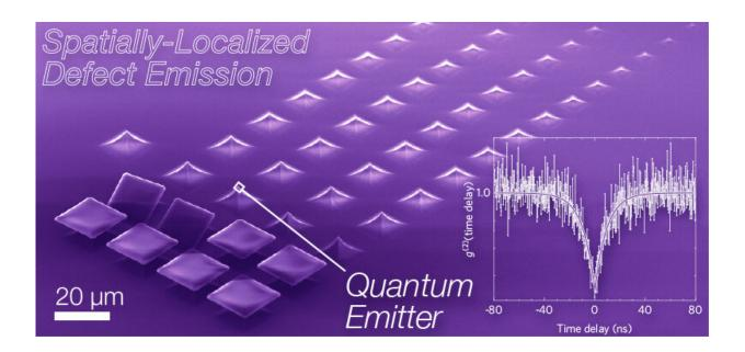
An innovative method for controlling single-photon emission for specific locations in 2D materials may offer a new path toward all-optical quantum computers and other quantum technologies. This image shows a false-color scanning electron micrograph of the array used to create place single-photon sources in epitaxial tungsten diselenide. Inset shows the Hanbury-Brown Twiss interferometry measurement proving quantum emission. Credit: Michael Pettes Los Alamos National Laboratory image
