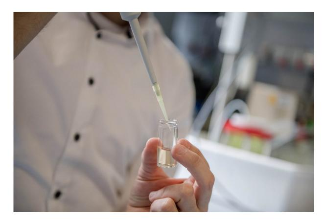
This solution contains the precursor material that is transformed into gold nanoparticles in the electrochemical experiments. Credit: RUB, Marquard
