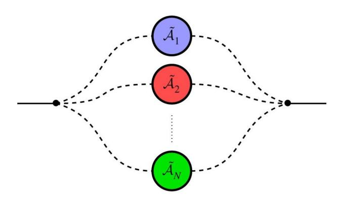
The superposition of N channels allows information carriers to travel through multiple channels simultaneously. Credit: Chiribella and Kristjánsson. ©2019 The Royal Society
