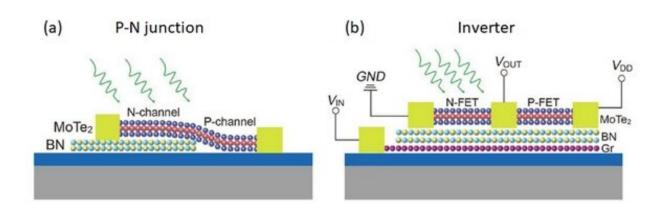
Figures (a) and (b) show the schematic illustration of a p-n junction and an inverter, respectively. Under light illumination and negative bias conditions, localized positive charges are left behind in the BN layer after the excited electrons travel into the MoTe2 layer. This induces doping effects in the MoTe2 layer. Credit: Advanced Materials
