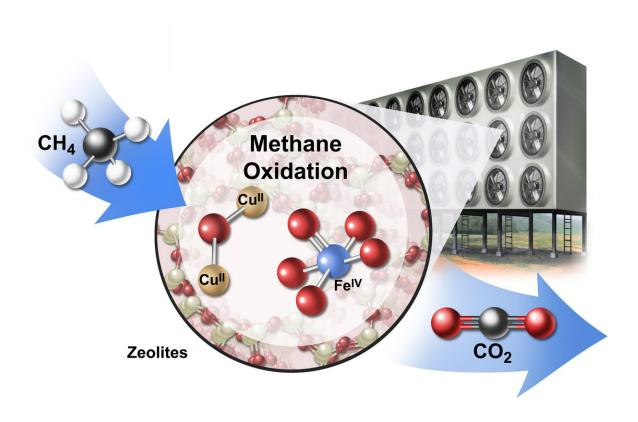
A conceptual drawing of an industrial array for converting methane (CH4) to carbon dioxide (CO2) using catalytic materials called zeolites (CUII and FEIV). Credit: Jackson, *et al.* 2019 *Nature Sustainability /* Artist: Stan Coffman
