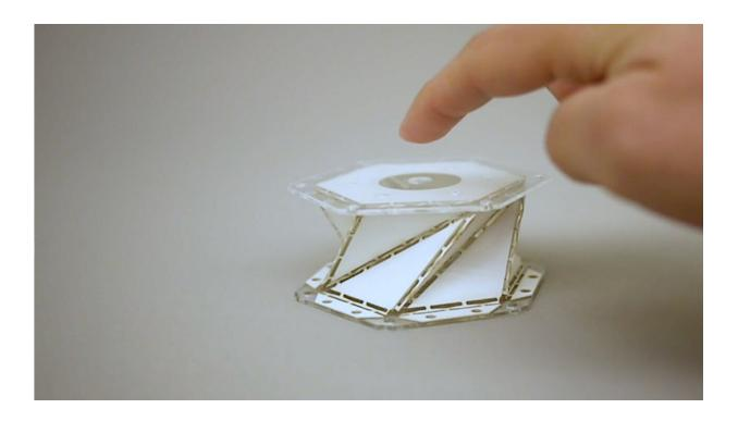
Inspired by the paper folding art of origami, a University of Washington team created a paper model of a metamaterial that uses 'folding creases' to soften impact forces for potential applications in spacecraft, cars and beyond. Credit: Kiyomi Taguchi/University of Washington
