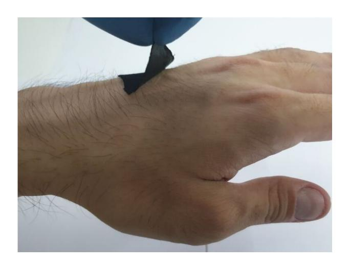
A graphene-based adhesive biosensor inspired by octopus "suckers" is flexible and holds up in wet and dry environments. Credit: Adapted from *ACS Appl. Mater. Interfaces* 2019, 11, 16951 16957
