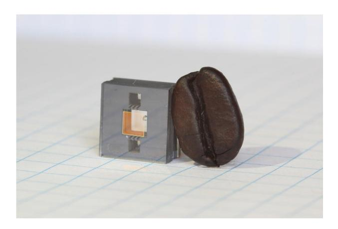
The heart of NIST's next-generation miniature atomic clock--ticking at high 'optical' frequencies -- is this vapor cell on a chip, shown next to a coffee bean for scale. The glass cell (the square window in the chip) contains rubidium atoms, whose vibrations provide the clock 'ticks.' The entire clock consists of three microfabricated chips plus supporting electronics and optics. Credit: Hummon/NIST
