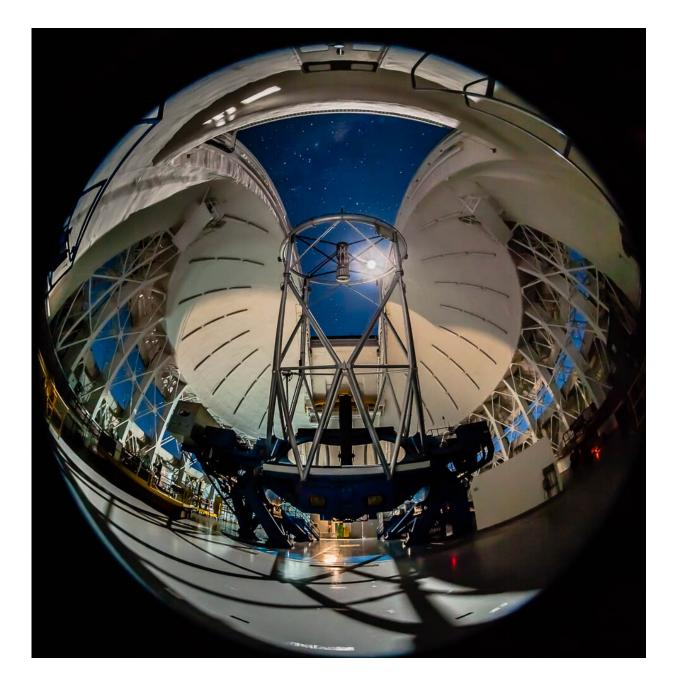
This stunning photograph taken, with a fish-eye lens from inside the Gemini South dome, shows the telescope nested in its altazimuth mount, pointing just high enough so that its monstrous 8-meter primary mirror is visible. Credit: Gemini Observatory/AURA image by Manuel Paredes
