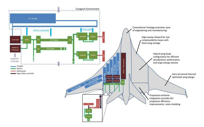
Concept sketch of a fully electric aircraft platform that uses cryogenic liquid hydrogen as an energy storage method. Credit: University of Illinois at Urbana-Champaign Department of Aerospace Engineering
