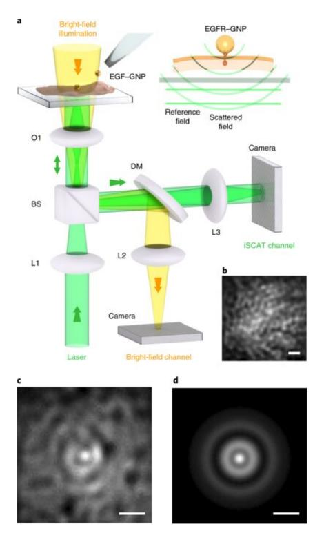
iSCAT microscopy on live cells. a, Experimental arrangement of the iSCAT microscope for live-cell imaging. Cells are plated in a glass-bottomed dish under Leibowitz medium. (a) micropipette delivers the EGF–GNP probes directly onto the cell culture, where they specifically target the EGFR protein in the cell membrane. The bright-field illumination channel from above assists in
