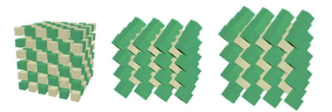
The zigzag packing is only observed for the body-centered tetragonal lattice (middle) and body-centered cubic lattice (right). In the simple cubic lattice (left), the nanocubes assemble face to face. Credit: Brookhaven National Laboratory
