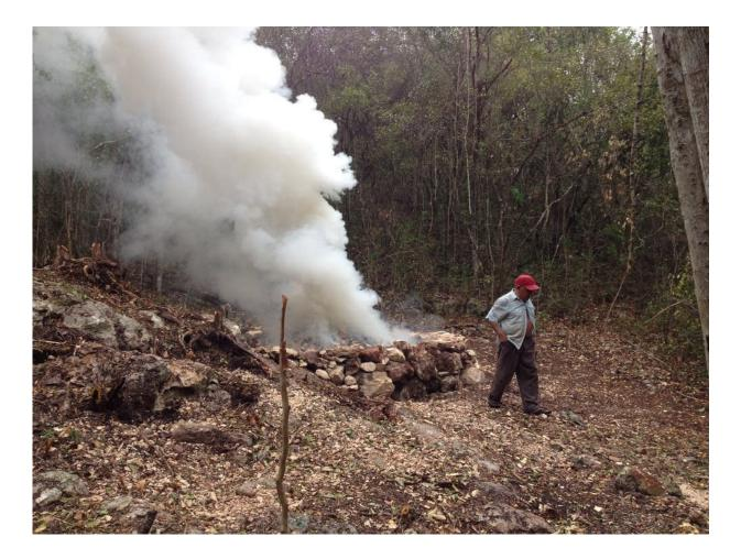
An experimental burnt lime pit-kiln, modeled on ancient pit-kilns excavated in the Northern Lowlands. Credit: Kenneth Seligson, <u>CC BY-ND</u>
