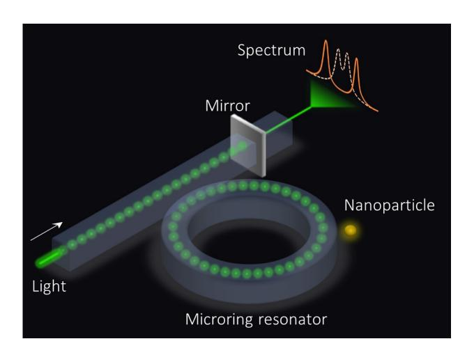
An exceptional surface-based sensor. The microring resonator is coupled to a waveguide with an end mirror that partially reflects light, which in turn enhances the sensitivity. Credit: Ramy El-Ganainy and Qi Zhong
