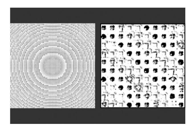
MIT mathematicians have developed a technique that quickly determines the ideal arrangement of millions of individual, microscopic features on a metasurface, to generate a flat lens that manipulates light in a specified way. The team designed a metasurface, at left, etched with millions of features. A zoomed-in image of the lens, right, shows individual features, each etched in a specific way so that, together, they produce a desired optical effect. Credit: Zin LIn
