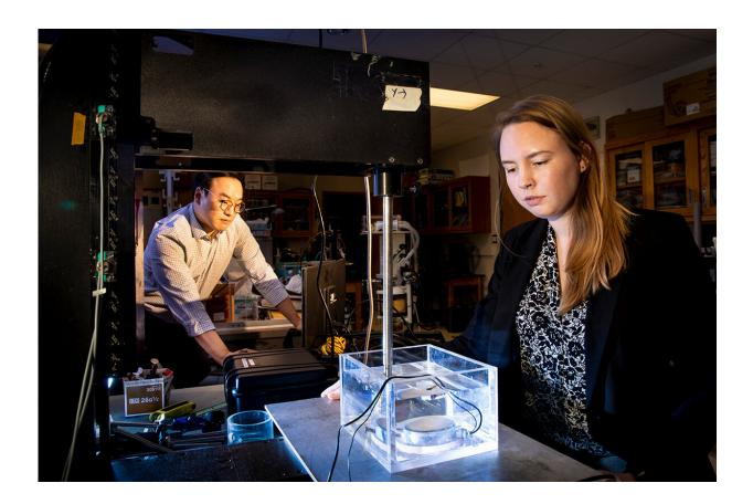
Gun Kim and Abigail Halmes work on equipment that emits an ultrasound wave inducing a reaction that produces light in synthetic molecules. Credit: Fred Zwicky
