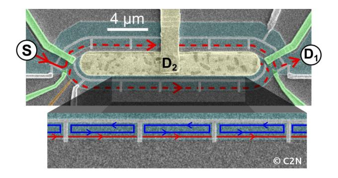
Colored scanning electron micrograph of the sample: Mach Zehnder interferometer and confinement strategy used to obtain and demonstrate a record electronic coherence length of 0.25~mm. Credit: © C2N
