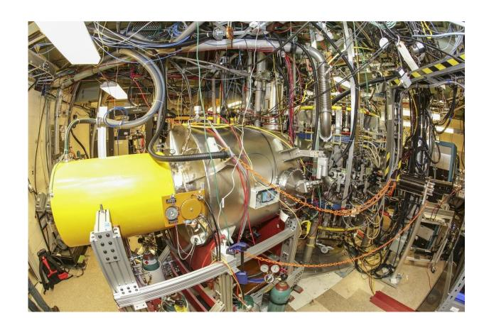
View of the LTX- $\beta$  with the neutral beam injector in yellow. Credit: Elle Starkman/PPPL Office of Communications
