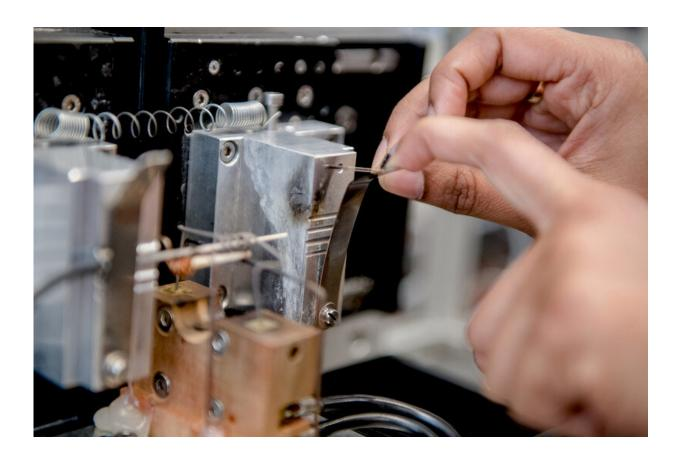
Invisible to the naked eye: at the tip of this carbon nanoelectrode the tiny catalyst particle is located. Credit: RUB, Marquard
