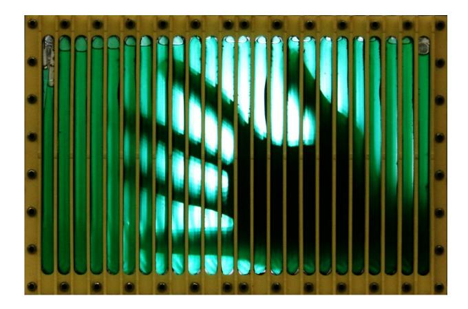
The Photobioreactor chamber is used to cultivate microalgae aboard the International Space Station in a demonstration of creating hybrid life support systems that use both biological and physicochemical processes. Credit: Institute of Space Systems - University of Stuttgart, Germany
