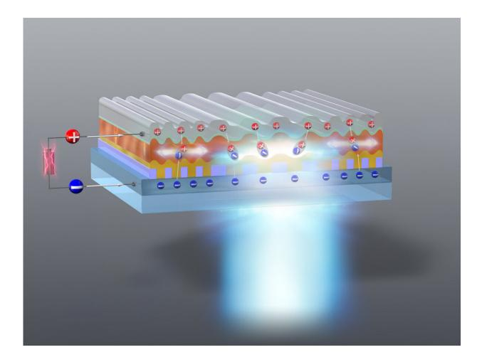
Schematic representation of an organic semiconductor laser diode producing blue laser emission under electrical excitation. Credit: Center for Organic Photonics and Electronics Research, Kyushu University
