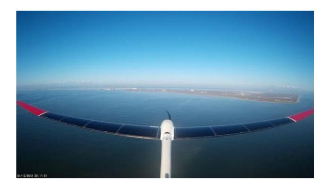
The Naval Research Laboratory is building solar-soaring drones that harvest energy from the sun and thermals to stay aloft for extended time periods. Credit: Naval Research Laboratory
