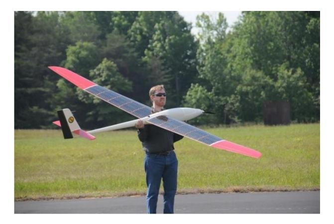
The US Naval Research Laboratory is designing long-endurance UAVs that use rising bubbles of warm air to stay aloft. Credit: Naval Research Laboratory
