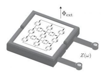
Josephson junction inside a microwave cavity, used to probe quantum behaviour via experiment. Credit: FLEET
