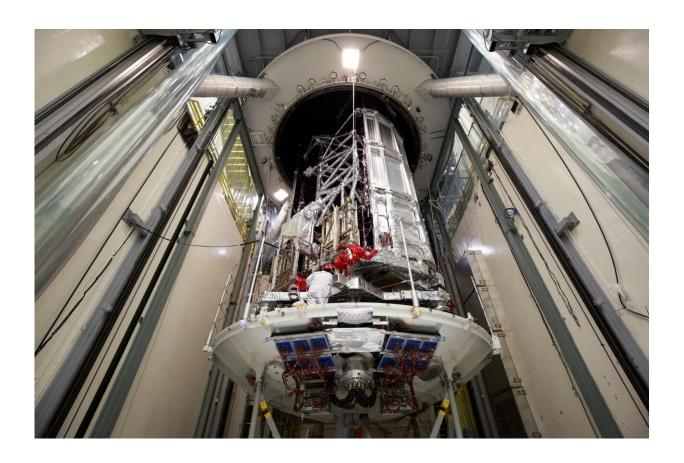
The James Webb Space Telescope's spacecraft element being prepared for entry into Northrop Grumman's large thermal vacuum chamber in Los Angeles, California. Credit: Northrop Grumman
