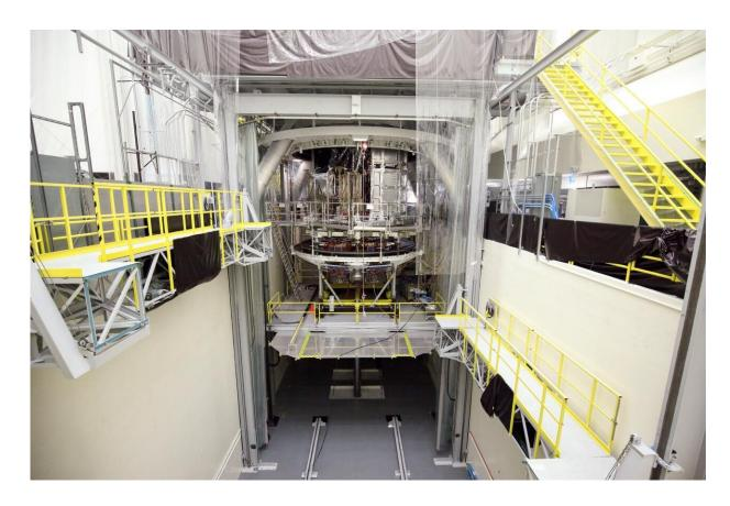
Webb's spacecraft being lifted into Northrop Grumman's thermal vacuum chamber for environmental testing to ensure that its hardware will function in the vacuum of space. Credit: Northrop Grumman
