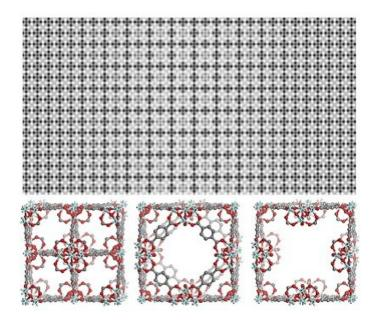
(Top) Processed high-resolution TEM image (top), showing coexistence of various defective structures in MOF UiO-66. (Bottom) Crystallographic models of three types of identified defects in MOF UiO-66. Credit: KAUST
